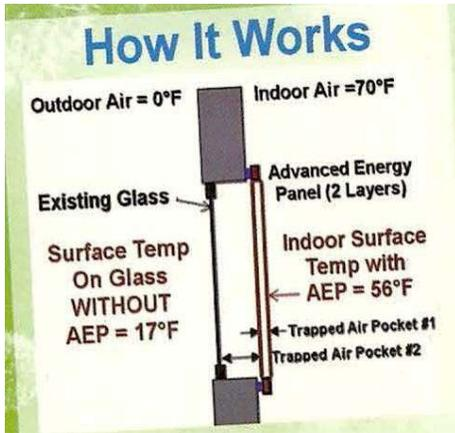
The graphic at left illustrates and quantifies the benefit— when it's 17° outside and 70° inside, the inside surface of the panels remains at 56°. With surface mounted to your window trim, the panels are guaranteed to stop condensation – because the warm air inside the building can't
